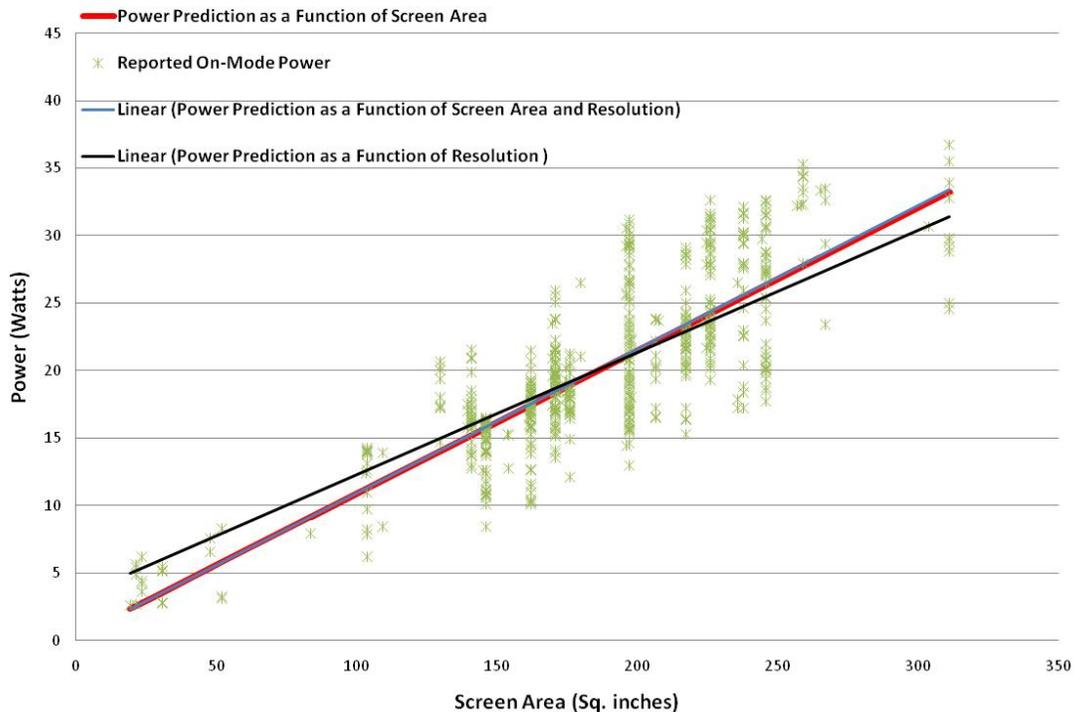
The variation between the power consumption prediction as a function of screen area versus as a function of both screen area and resolution is only about 2 percent, with a mean absolute error of 0.05 watts. The relationship between these two approaches is illustrated for nine randomly selected models in Figure 2. Note that all of the selected models would have qualified for ENERGY STAR had the calculation for maximum On Mode power consumption been based only on screen area.
