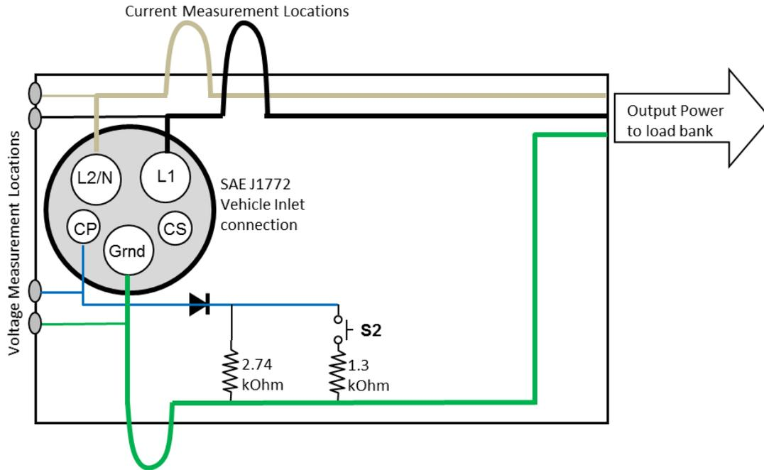
**Figure 3: Schematic of Vehicle Emulator Module (VEM)<sup>2</sup>**
