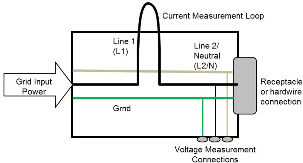
**Figure 2: Schematic of Input Measurement Apparatus (IMA)<sup>1</sup>**
